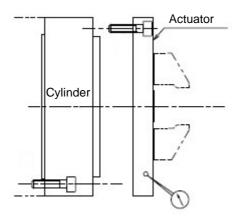
Attach the actuator and then check that it is centered to a deflection of no larger than about 5 microns.
