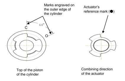
Normal: The cylinder's engraved mark (C) and the actuator's mating mark (●) are engaged at the identical position.
