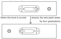
In this case, adjust the position of the bubble by turning the adjusting screw until the bubble moves back by two graduations (a half of the variation).
