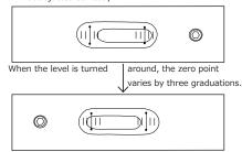
In this case, adjust the position of the bubble by turning the adjusting screw until the bubble moves back by 1.5 graduations (a half of the variation).
