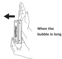
Face up the zero point adjusting screw and tap the back side of the zero point adjusting screw (measuring plane).
