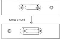
The right side of the surface plate is two graduations higher than the left side.
