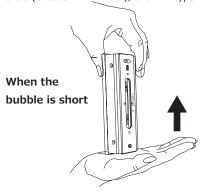
Face down the zero point adjusting screw and tap the side of a level. Small bubbles rise and therefore the main bubble is lengthened.
