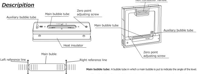
Main bubble tube: A bubble tube in which a main bubble is put to indicate the angle of the level. Auxiliary bubble tube: A bubble tube that indicates an inclination in the Y-axis direction. Zero point adjusting screw: A screw used for zero point adjustment of a level (centering of the main bubble) before use.
